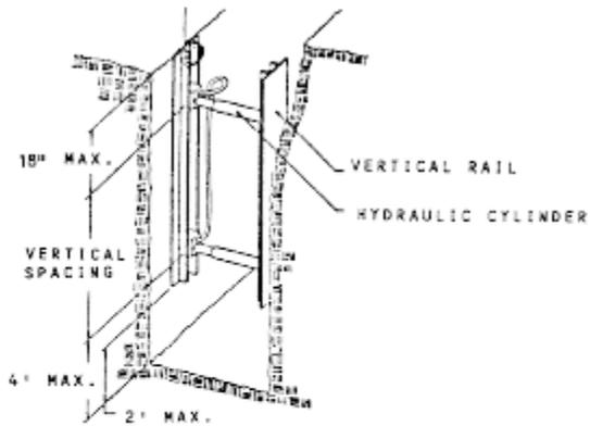
Figure 2. Pneumatic/hydraulic Shoring
