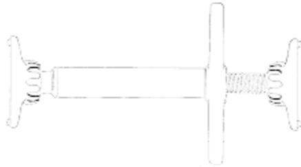
Figure 4. Trench Shields
